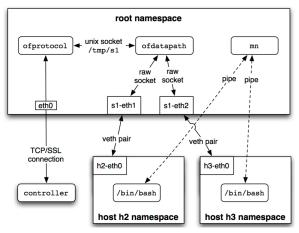
Mininet creates a virtual network by placing host processes in network namespaces and connecting them with virtual Ethernet (veth) pairs. In this example, they connect to a user-space OpenFlow switch.
