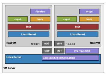
OK, but VMs are heavyweight: the memory overhead for each VM limits the scale to just a handful of switches and hosts.
