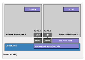
Mininet leverages Linux features (processes and virtual Ethernet pairs in network namespaces).
